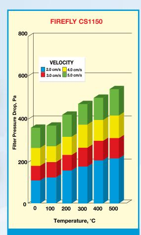
The clean filter pressure drop is dependent upon the filter face velocity and operating temperature. TENMAT filter elements exhibit a uniquely low pressure drop with respect to velocity and temperature, and this is illustrated on the graph.
